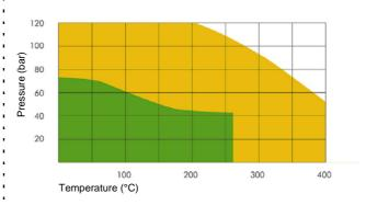
The P x T diagram above indicates the service limits for NA-1100 considering the simultaneous influence of pressure and temperature (chemical suitability assumed). The green area represents the normal service limits, while the orange coloured area shows the maximum application limits. For those cases, please consult our technical department.
