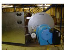
Containerised and skid mounted packaged boiler units and ancillary equipment assembled in our works and dispatched to site fully tested and ready for connection to the system.
