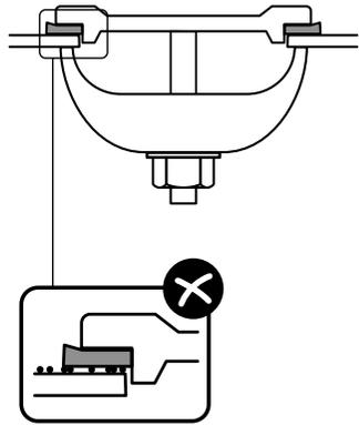
3. Gaskets on the bottom of a boiler shell are typically more difficult to install without leaking because small particles tend to become lodged between the mating surfaces after they have been cleaned. This can lead to over-tightening of the gasket to stop leakage. It is recommended to drain the boiler and start over or the gasket's service life may be shortened.
