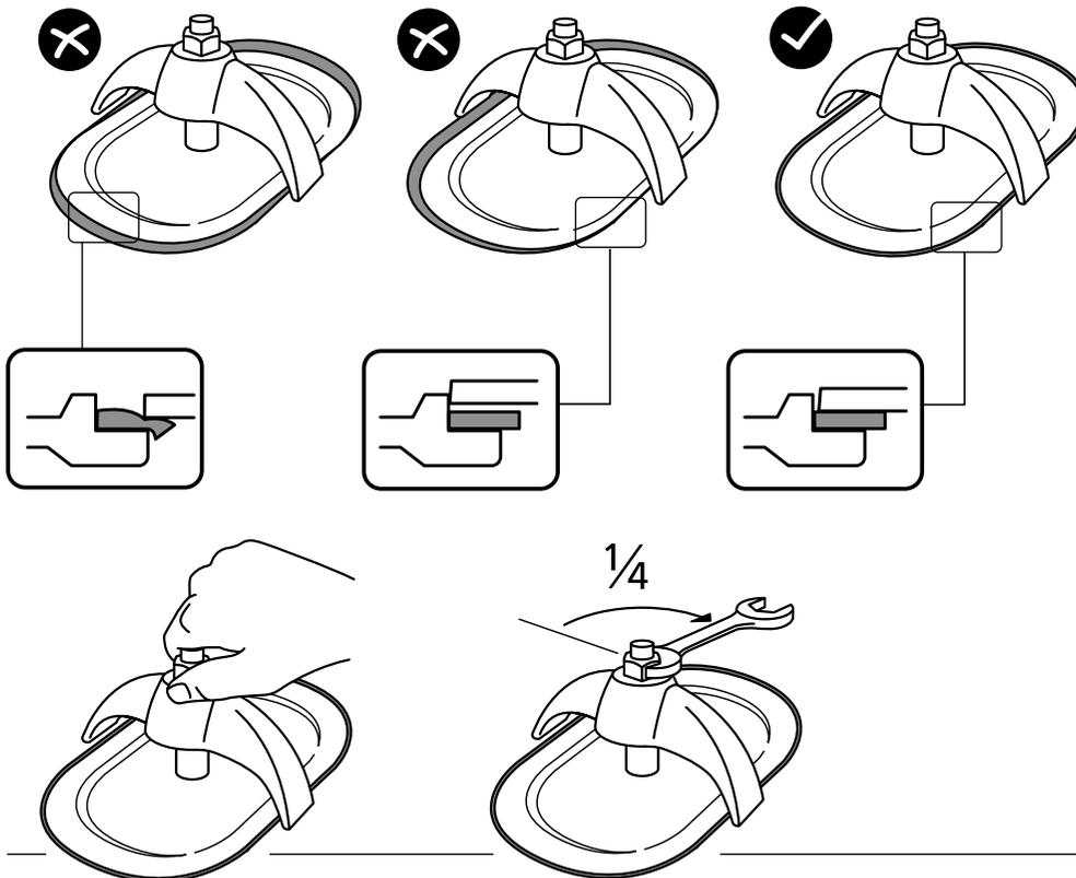
2. Set crab, then center plate in opening and tighten nut enough to give a snug fit. Make it hand tight then increase pressure on the gasket with a quarter turn of wrench.
