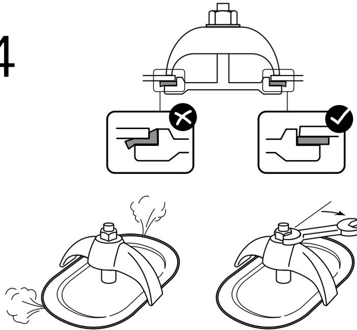
4. Do not over-tighten as it will over-compress the gasket and shorten its service life.
