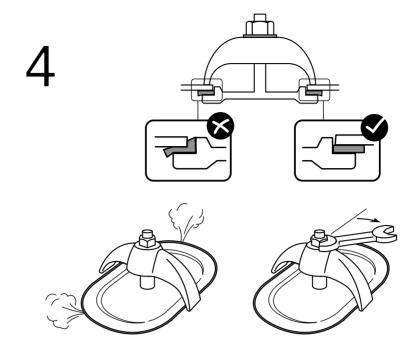
4. Do not over-tighten as it will over-compress the gasket and shorten its service life.
