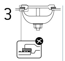
3. Gaskets on the bottom of a boiler shell are typically more difficult to install without leaking because small particles tend to become lodged between the mating surfaces after they have been cleaned. This can lead to over-tightening of the gasket to stop leakage. It is recommended to drain the boiler and start over or the gasket's service life may be shortened.
